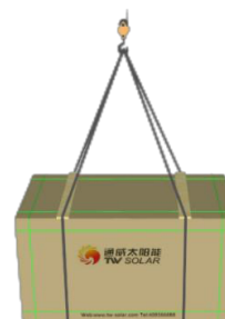
Figure 6 Schematic diagram of Module lifting
